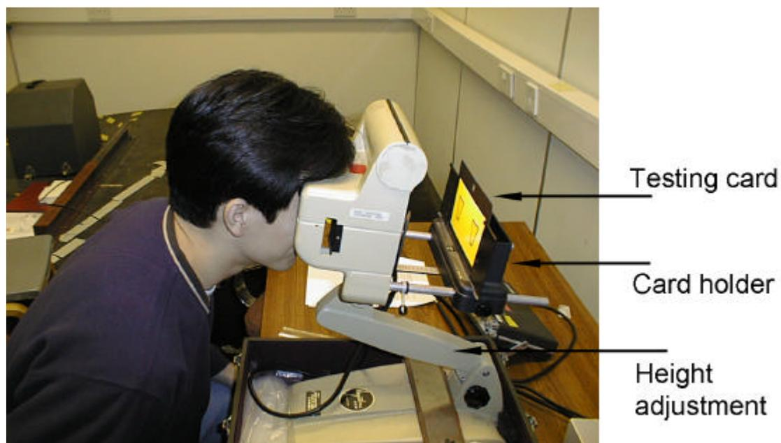
**Figure 3.5.** A subject undergoing vision tests with the Keystone visual skills profiles testing equipment. Card holder is set to the ‘far point’. The holder can be moved towards the subject to the ‘near point’.
